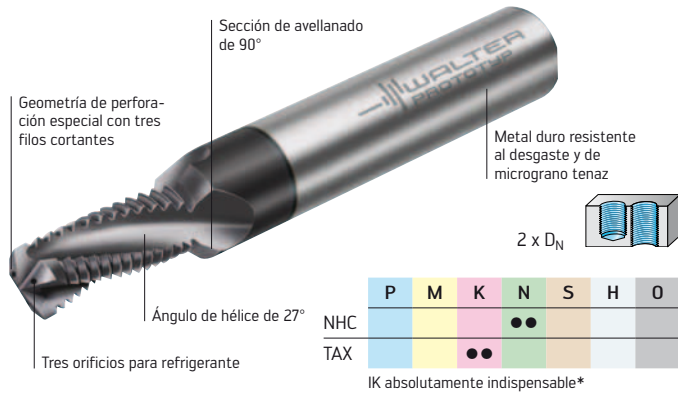
Fresa de roscar MDI TMD - Thread Mill Drill
