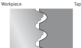
Axial miscutting of the thread caused by right-hand helical tools: miscutting of the bottom face of the flank
