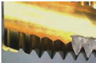
Example of fractures due to chip control problems
