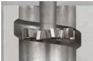
Inclination P = 12 – profile is distorted
