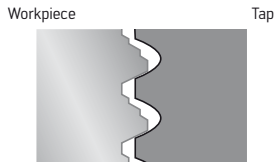
Axial miscutting of the thread caused by left-hand helical taps or taps with a spiral point: miscutting of the top face of the flank
