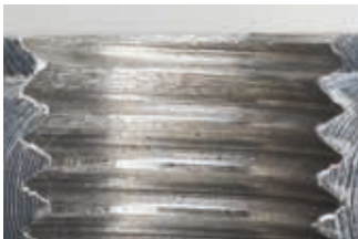
Axially miscut blind hole threads
