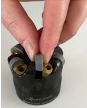
① Insert the ceramic indexable insert Note the direction of cut!
