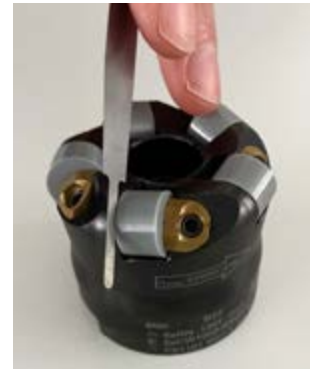
④ Check that the indexable insert is securely fitted
