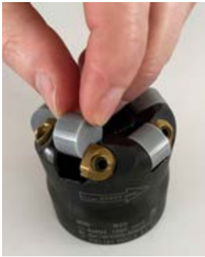
① Insert the ceramic indexable insert
