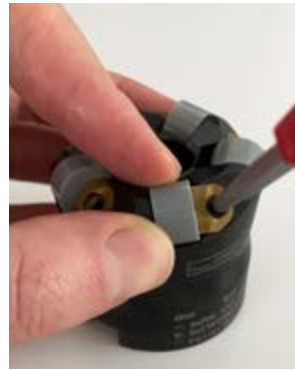
③ Secure the ceramic indexable insert
