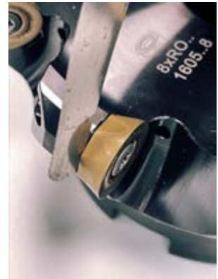
④ Check that the indexable insert is securely fitted
