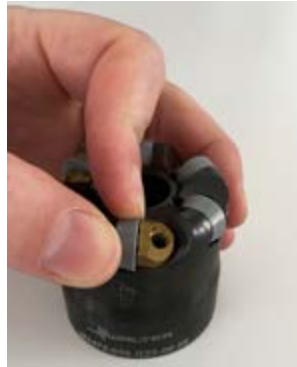
② Fit the ceramic indexable insert
