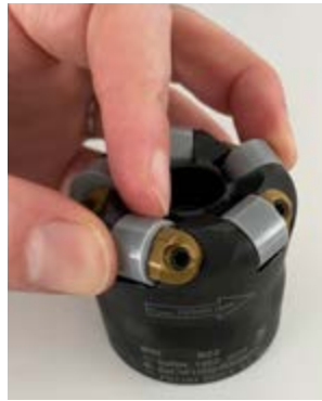
② Fit the ceramic indexable insert
