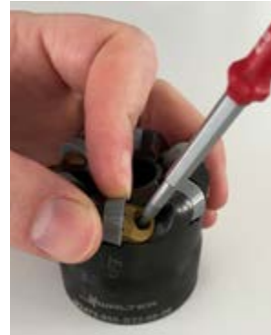
③ Secure the ceramic indexable insert
