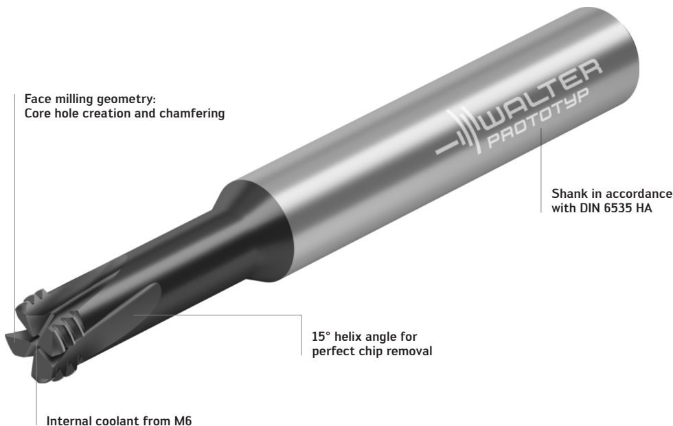
Solid carbide orbital drill/thread mill
