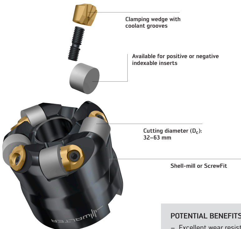
New milling cutter for button ceramic inserts
