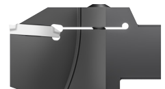
Adapted cutting depths: 0.196-1.299 in (5–33 mm)
