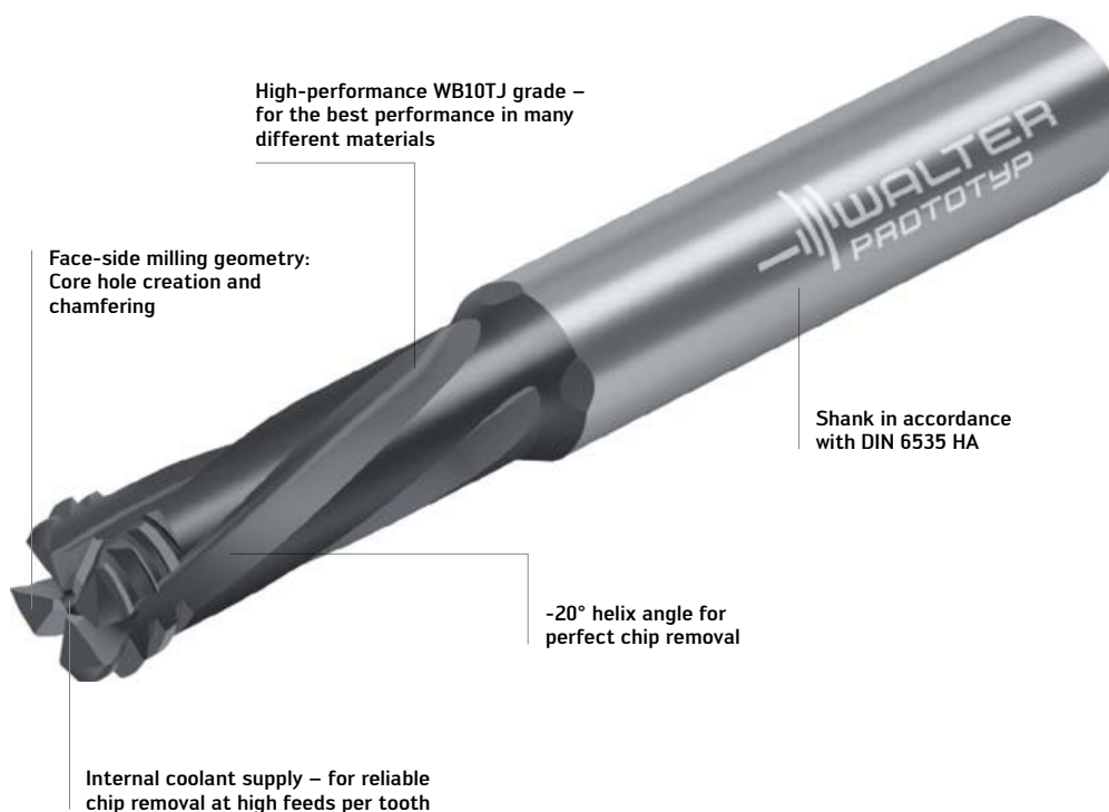
Solid carbide orbital drill/thread mill
